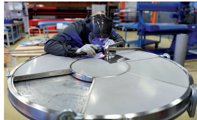
Welded composite discs up to 3 metres in diameter
