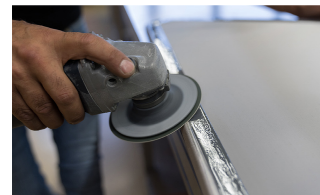
The filter frames are then hand finished before being delivered back to our customers.
