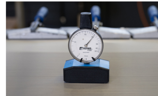
Meshes are tensioned to the required levels and attached to the frames. Our extensive experience ensures that the meshes will not lose tension over time.
